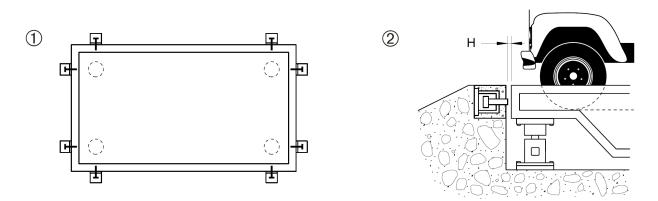
Using accessories **72903** - **72904** the platforms admit the use of tie rods or stoppers. If stoppers are used ① it must be left a maximum spread ② of: H<6 mm. We recommend to clean and to grease periodically the internal balls.
