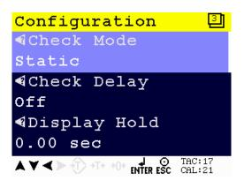
When pushing the LEFT key, the help text of the parameter is shown.
