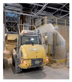
Fig. 2 The lift truck on the floor scale to determine the tare waight
