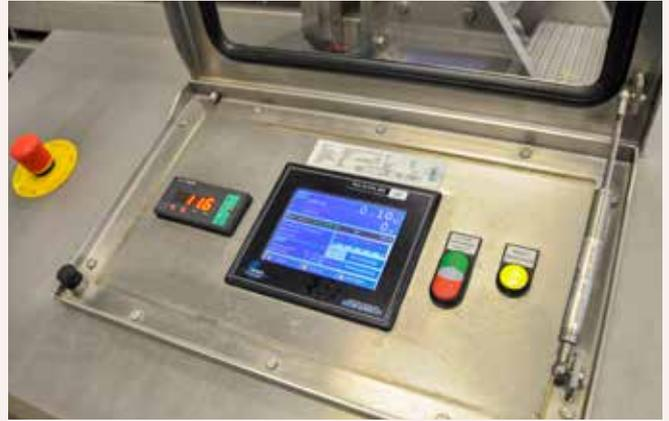
△ Two stainless steel bulk tanks with the corresponding filling controller.. at the right : eThe control desk with a FLEX filling controller.
