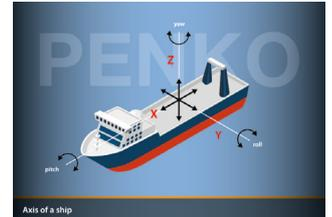
Picture 1. The movements of a ship, caused by the waves, around the three axis.
