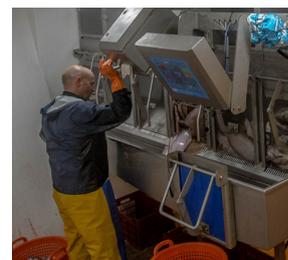
*Photo 4. A platform weigher on which the catch is packed in buckets.*
