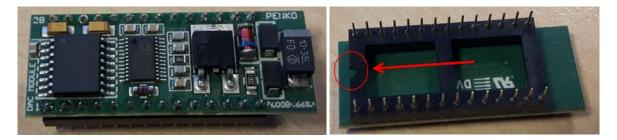
This mark needs to line up with the mark on the 1020 circuit board.
