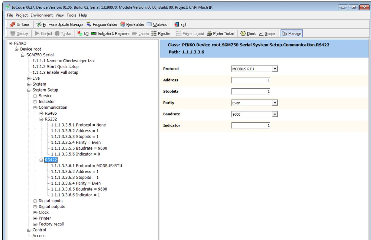
The screenshot displays the PENKO software interface. The left pane shows a tree view of the device configuration. The right pane shows the configuration for the selected 'RS422' communication method. The settings are as follows:
