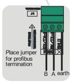
Main board revision F or higher has a double dip switch for Profibus termination
