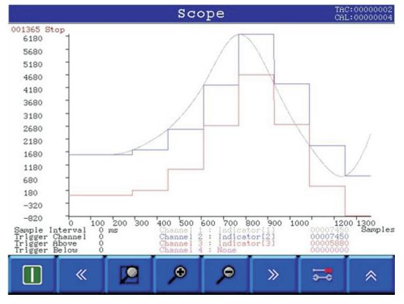
In this example the sample rate is set to the maximum of 1600 samples/sec by setting the interval to 0ms. Under system setup->Indicator setup-> indicators the different indicators have been setup:
