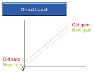
Its also possible to change the line position if there is weight on the scale. To do so, edit the actual weight value to the new known value.
