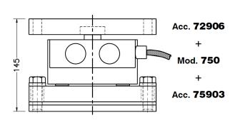
Accessory lower plate is permanenty fixed to the structure or ground by welding or cement. Unscrew the upper plate it's enough, to replace a load cell.
