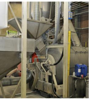
rature. Should the temperature increase over a specified set value, the system will automatically stop the dosing of the ammonia until the mixture has cooled down to the set value. This cycle is repeated until the required amount of ammonia has been added. After completion of the blending time, the mixture is transported to an interim storage.
