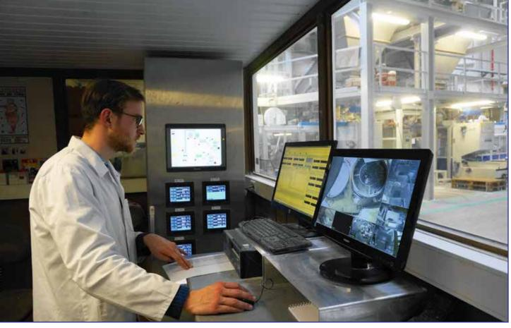
Washing-powder Production Separate controllers instead of one PLC control for all weighing systems improves weighing accuracy
