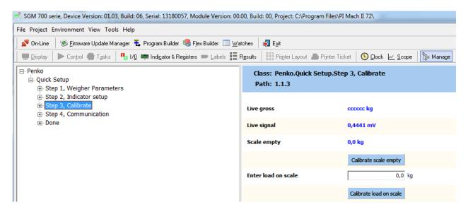
Make sure the weighing installation is empty. Click on Calibrate scale empty.
