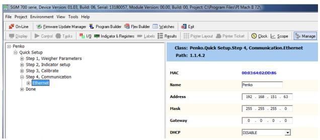
The SGM7xx/SGM8xx can have an Ethernet, CAN bus, Profibus or Serial output, depending on which version you have.
