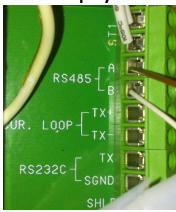
Connect **pin 1** of the FLEX or FLEX 2ch. - 4ch. sub-D connector to **RS485-B** on the display, and connect **pin 9** of the FLEX or FLEX 2ch. - 4ch. sub-D connector to **RS485-A** on the display.
