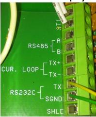
Connect **pin 3** of the FLEX or FLEX 2ch. - 4ch. sub-D connector to **RS232 TX** on the display, and connect **pin 5** of the FLEX or FLEX 2ch. - 4ch. sub-D connector to **RS232-SGND** on the display.
