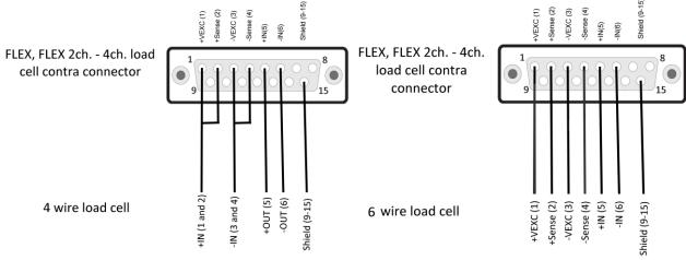
Note: when you use a 4 wire load cell, +IN <u>must</u> be connected to +VEXC <u>and</u> +Sense.
