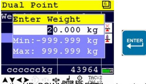
Use the UP, DOWN and LEFT key to enter the reference value. The UP and DOWN keys are used for changing the number (1-9), the LEFT key is used for changing the position of the cursor.
