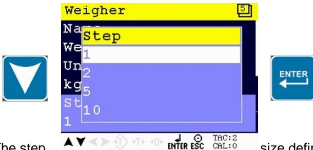
The step size define the scaled parts of the weigh value. The display value will be rounded off to the nearest value with a valid step size. Step size can be 1, 2, 5, 10, 20, 50,100, 200.
