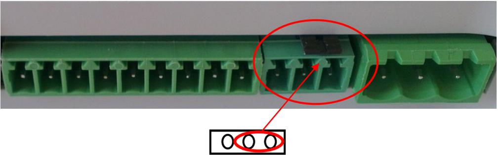
Jumper setting termination on (120 Ω)
