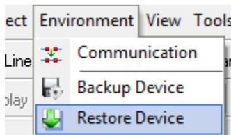
An open dialog is shown. Select the backup file, and click OPEN. The image will be programmed into the device, and the device will restart.
